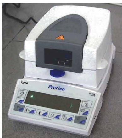
Moisture Measurement Test
