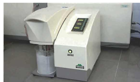
Grain Thickness Distribution Measurement Test
